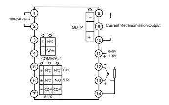
Note: Linear voltage signal of range below 1V should be inputted from terminals 13 and 12, and signal of  $0 \sim 5V$  and  $1 \sim 5V$  should be inputted from terminals 11 and 12.  $4 \sim 20$ mA linear current signal can be converted to  $1 \sim 5V$  voltage signal with a 250 ohm resistor and inputted from terminals 11 and 12.
